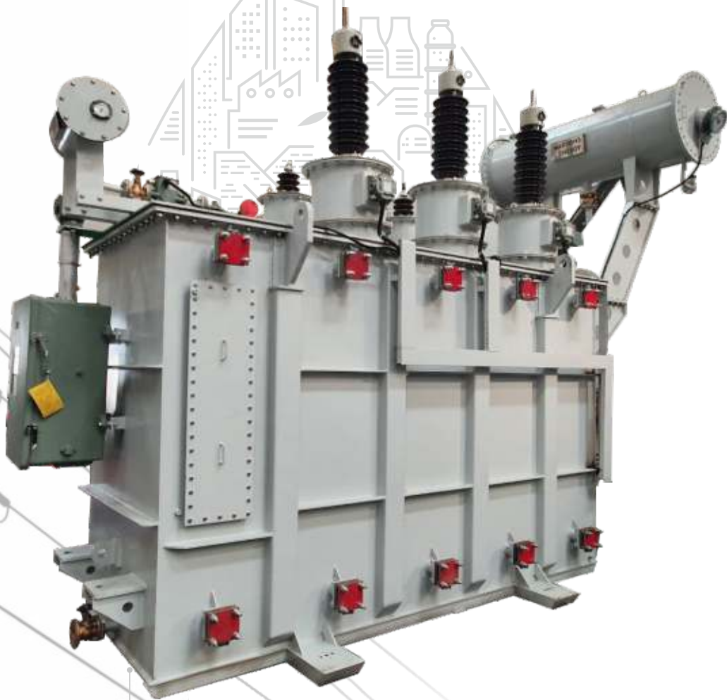
10 MVA, 6/11 kV, ONAN, Copper Wound Power Transformer with MR G&many Make On Load Tap Changer
