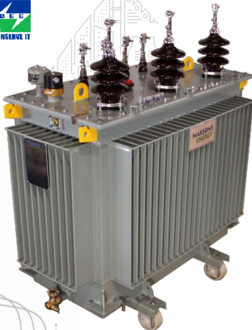
500 kVA, 11/0.433 kV, ONAN, Copper Wound Hermetically Sealed Distribution Transformer with Off Load Tap Changer
