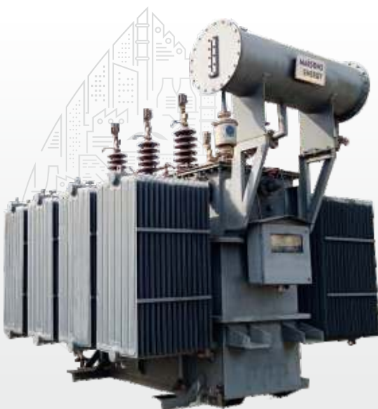
5 MVA, 33/11 kV, ONAN, Copper Wound Power Transformer with Off Load Tap Changer
