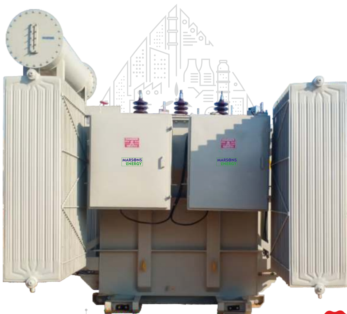
5 MVA, 0.800-0.800/33 kV, ONAN, Copper Wound, 3 Winding Inverter Duty Transformer with Off Load Tap Changer
