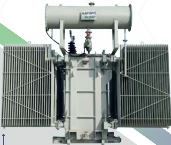
6 MVA, 0.800-0.800/33 kV, ONAN, Copper Wound, 3 Winding Inverter Duty Transformer with Off Load Tap Changer Evacuation Substation 45 MW Solar Farm
