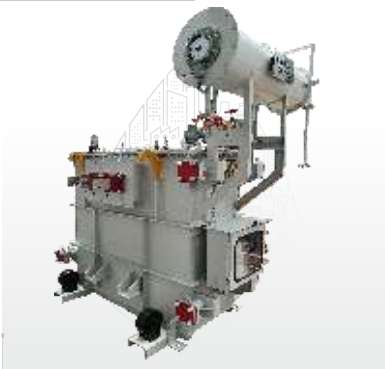
2.5 MVA, 0.630-0.630/33 kV, ONAN, Copper Wound, 3 Winding Inverter Duty Transformer with Off Load Tap Changer
